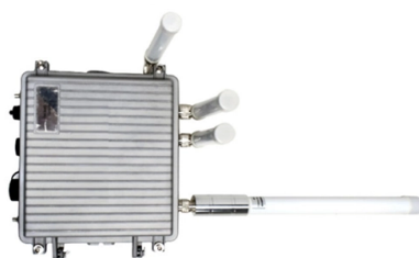
LoRawan outdoor base station
